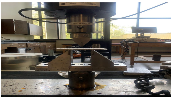
3-Point Bending Test Set-up
