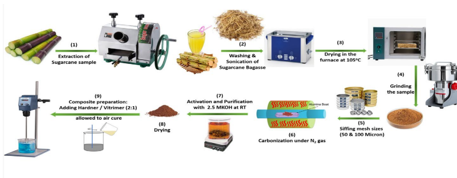
Overview of natural fiber treatment & Laminate Formation
