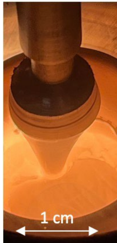
Figure 2: Modified Czochralski technique shown. CoCrFeNi single-crystal boule is being grown/pulled in an RF furnace. Seeding W single-crystal rod shown at top.
