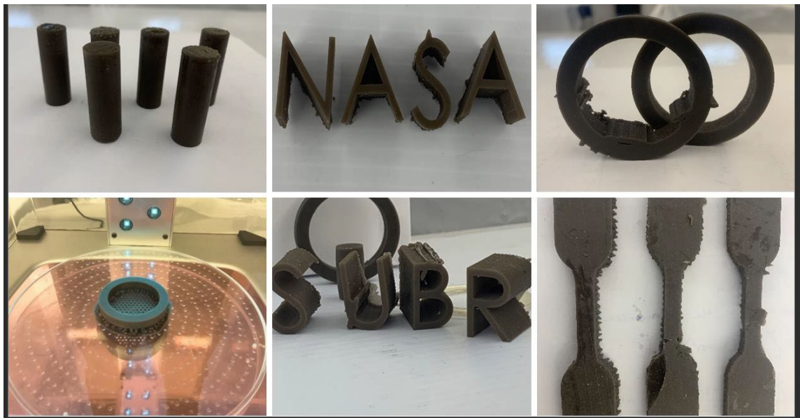
Figure 1. 3D printed SMV-regolith composite samples using digital light processing (DLP) printer.
